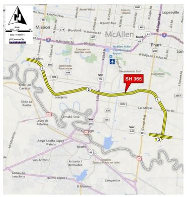
SH 365 consists of three phases of construction of toll and non-toll improvements of independent utility from FM 1016 / Conway Ave to US 281 / Military Highway for project length of 17.4 miles between two crucial port of entry within Hidalgo County (Anzalduas Bridge and Pharr-Reynosa International Bridge).
